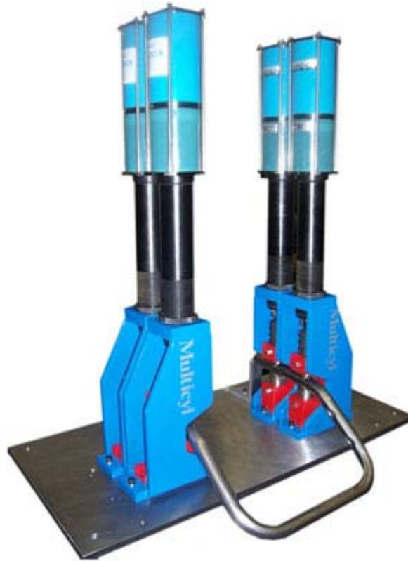
An application in which the customer used four H2 Multicyl units in a tube piercing cell.
