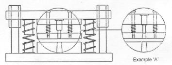
Do not attach tooling directly to the ram.
