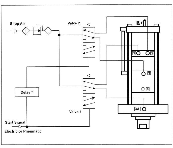
**Pneumatic Circuit for Power Boost Cylinders**
